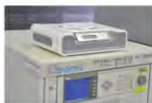
Power Input Tolerance Testing
